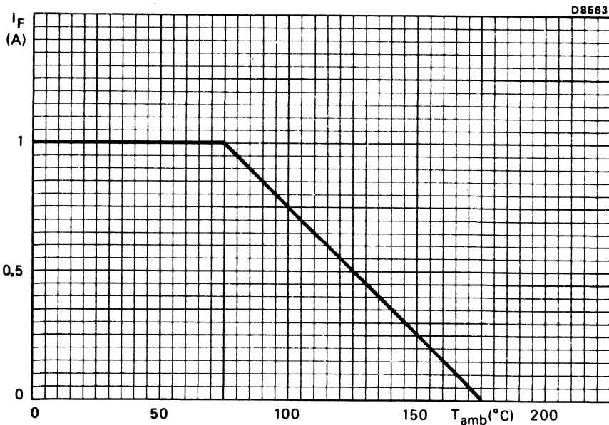
Fig.4 Maximum permissible d.c. forward current
